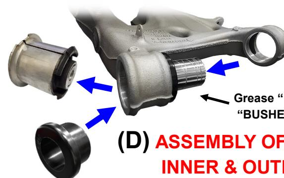
(D) **ASSEMBLY OF THE (4) NEW INNER & OUTER BUSHINGS**
